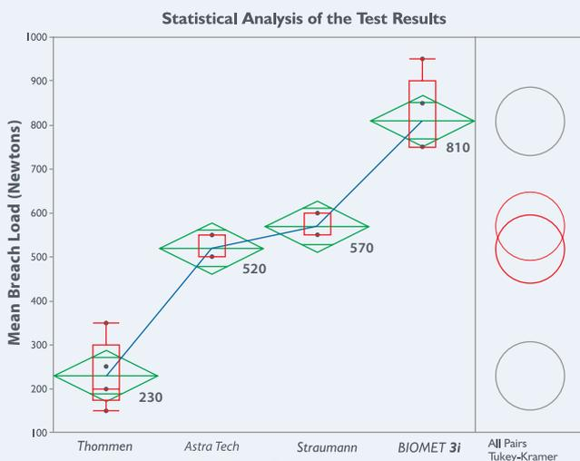
Fig. 2. Statistical analysis of the test results for the four implant groups in the study.
