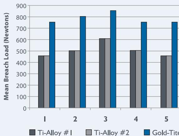
Fig. 3. Breach Load (N) for the BIOMET 3iT3® Implant and GingiHue® Abutment with either a Ti Alloy or Gold-Tite® Abutment Screw.
