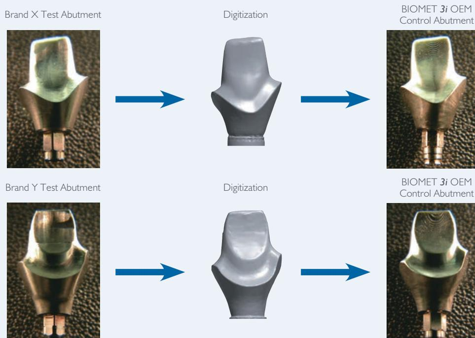
**Fig. 6.** Utilization of the copymill process enabled the investigators to create "control abutments" (possessing the OEM connection) with equivalent external geometry to the aftermarket "test abutment."
